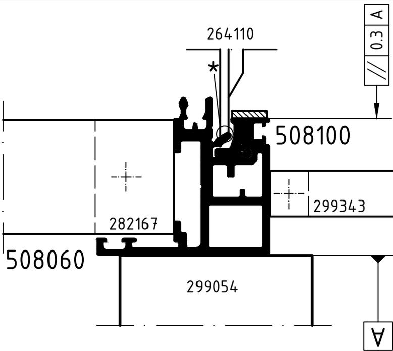
\*Attention! Set the pressure from above as follows: Set F1 so that you touch the profile shell 508290 lightly and then remove F1. Low lateral pressure!  $R_{usv} = 10-20 \text{ N/mm}$ .
