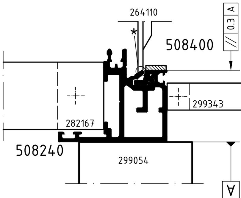
**\*Attention!** Set the pressure from above as follows: Set F1 so that you touch the profile shell 508290 lightly and then remove F1. Low lateral pressure!  $R_{usv} = 10-20 \text{ N/mm}$ .
