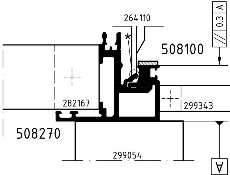
**\*Attention!** Set the pressure from above as follows: Set F1 so that you touch the profile shell 508290 lightly and then remove F1. Low lateral pressure!  $R_{usv} = 10-20 \text{ N/mm}$ .
